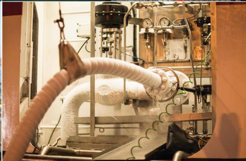
**Cryogenic Break-away Couplings** are a further development of our Safety Break-away Couplings which has successfully been used to prevent pull-away accidents in the petroleum, chemical and LPG industry all over the world. The new range of Cryogenic Break-away Couplings can be installed either at fixed points or in the middle of hose strings.
